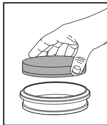
6. Allow filter to dry for 24 hours before putting back into the vacuum cleaner.
